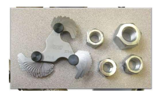
Thread pitch can be determined using a pitch gage or with nuts that you know the size and pitch. You can also measure one inch and count the number of threads in that one inch section.
