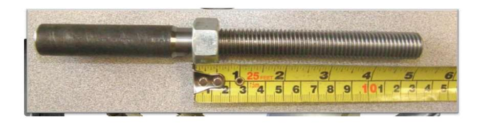
Thread length is measured to the end of a nut that is threaded all the way up the threaded portion of the threaded stud.
